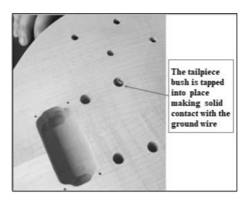
Installing the tailpiece bushing may be done with a plastic headed mallet or place a small piece of wood on top of the bushing to prevent damage and top the bushing in place with an ordinary hammer. Now screw the tailpiece mounting screws back into
