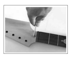
tightening the truss rod adjustment nut that protrudes from the base of the headstock just above the nut. A "back bow" or "hog-back" can be removed by loosening the nut. Great care should be taken with truss rod adjustments where as little as 1/4 of a turn can vastly alter the shape of a neck. A broken truss rod of course means a costly replacement.
