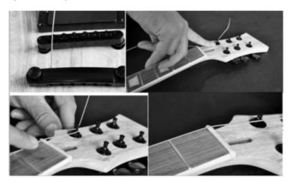
Now adjust the height of the strings over the 12th fret. Adjustments to the string action are made by raising or lowering the bridge with the thumbwheel height adjusters (LP) or by adjusting the single brackets (Tele, Strat-style, JB-Bass). Following is a chart to assist you. This action adjustment is a matter of personal preference. There should be a gradual increase in height from the first to the sixth (forth) string.
